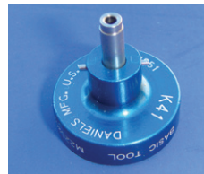
Figure 4: Socket positioner (K41)
