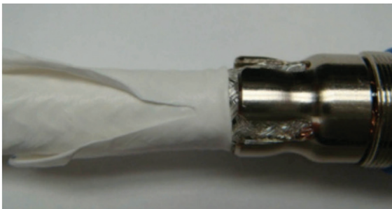
Figure 22: Returning the outer jacket
