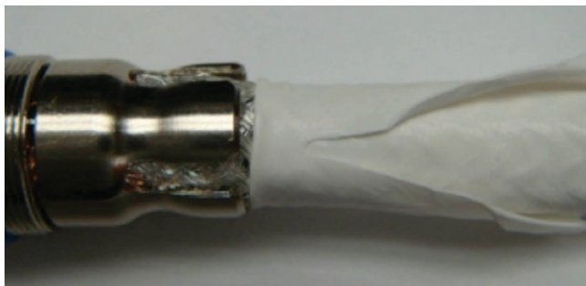
Figure 39: Returning the outer jacket
