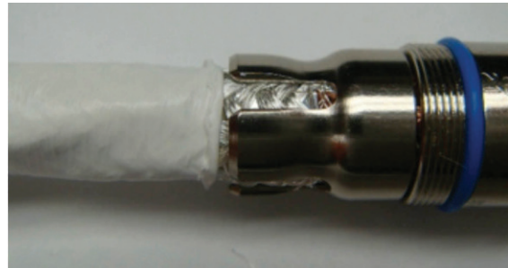
Figure 23: Trimming the outer jacket
