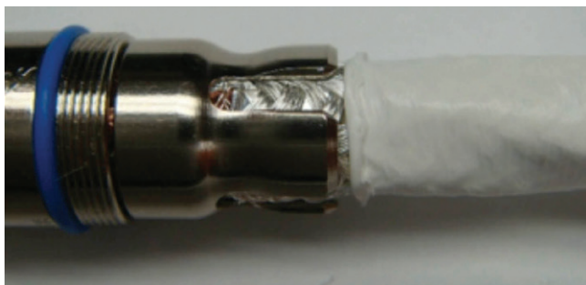
Figure 40: Trimming the outer jacket
