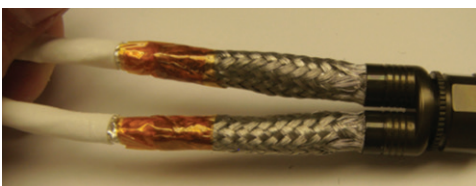
Figure 47: Taping the braid
