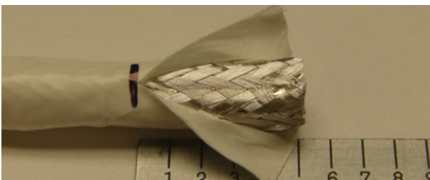
Figure 16: Slitting the cable jacket
