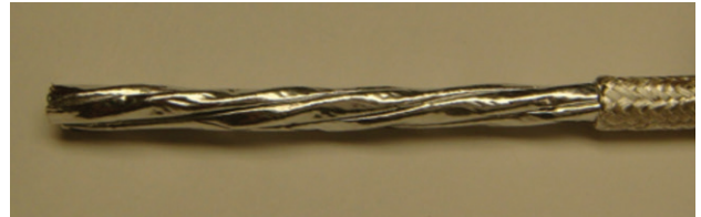
Figure 18: Exposing the foil
