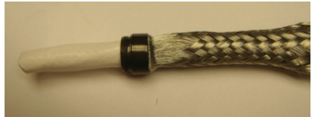
Figure 30: Inserting cable into braided shield
