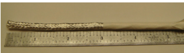
Figure 17: Exposing the braid
