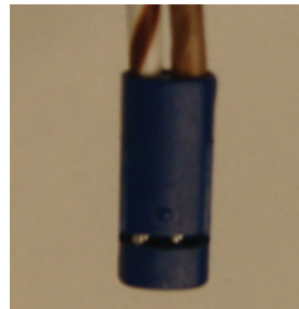
Figure 25: Inserting pair into plug insulator
