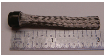
Figure 12: Cutting bottom insert braid shield
