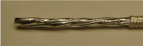
Figure 34: Exposing the foil
