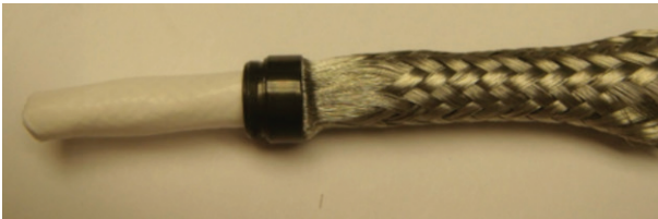
Figure 14: Inserting cable into braided shield
