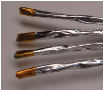
Figure 35: Wrapping the foil
