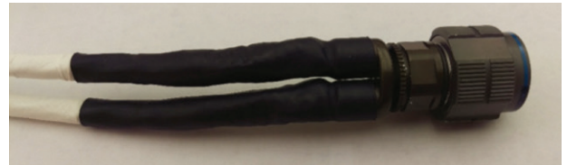
Figure 49: Covering the plug with TAT material
