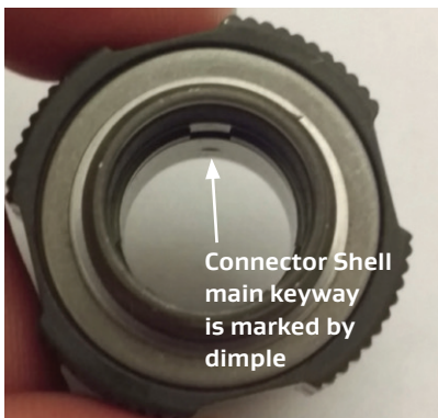
Figure 29: Inserting connector shell on cable
