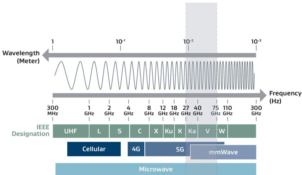
2. DoD utilization of mmWave frequencies comes in the Ka-band from 27 to 40 GHz and V-band from 40 to 75 GHz.
